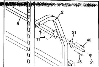
6. Press a 25mm Round Inner Cap (51) into the end of the other Weight Storage Tube (21).
